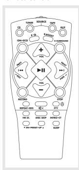
**ON-ECO** — keep pressing briefly **STANDBY** mode to enter ECO (power saving, without clock display) mode.
